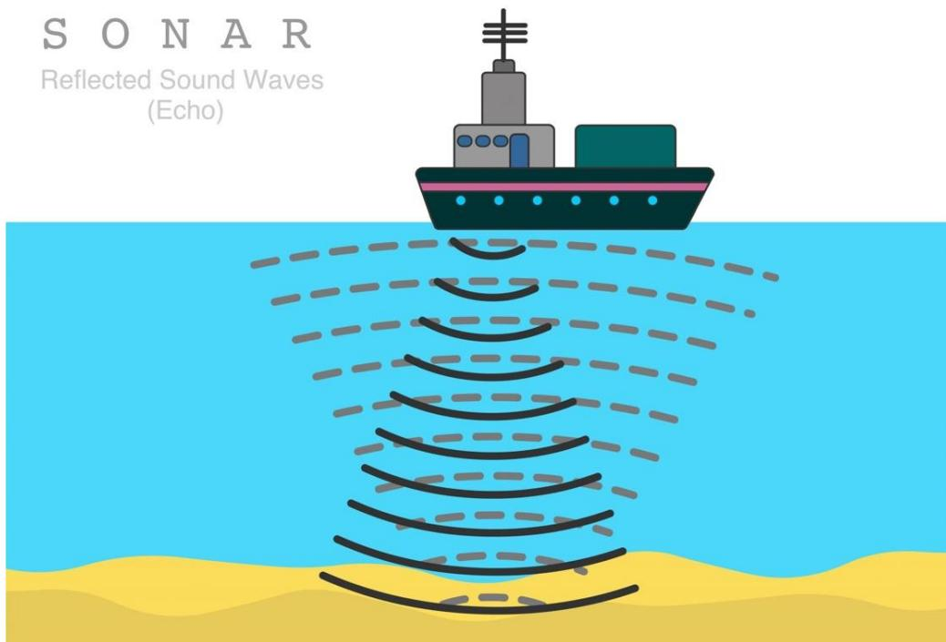
**Slika 1. Princip odašiljanja i zaprimanja signala sonara. Izvor <https://www.americanoceans.org/facts/what-is-sonar/> [3]**
